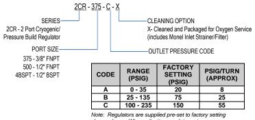
Note: Regulators are supplied pre-set to factory setting shown above. When adjusting regulator set pressure up (CCW) or down (CCW), approximate PSIG/TURN can be used as a reference.
