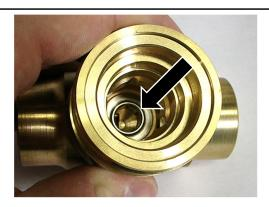
3.) Inspect the Valve Seat for any damage and replace if necessary (see step 3a).
