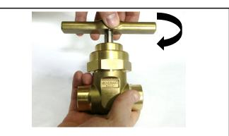
6.) Remove handle and replace bonnet. Tighten bonnet to 80 ft·lbs. Replace Handle and actuate valve to ensure smooth operation.
